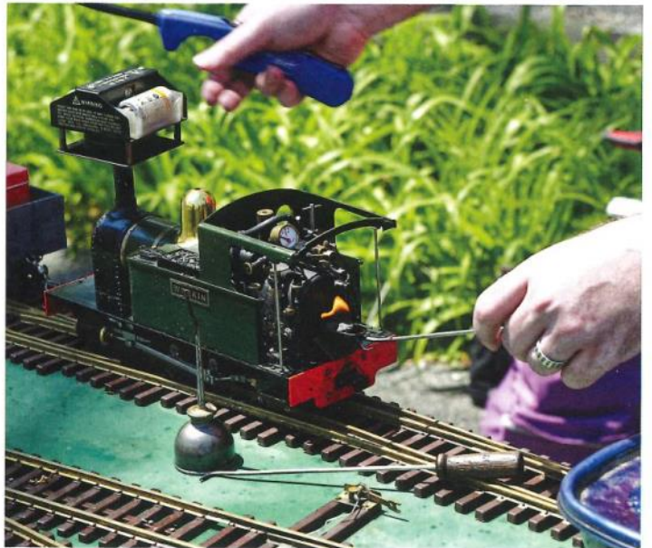
The author lights the fire in his coal-fired 0-6-0, which started life as a basic Accucraft Wrekin before alterations like a new boiler and axle pump were added.
